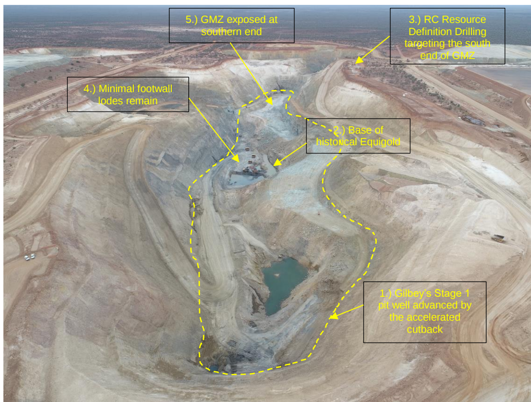
Figure 1b: Highlights the key aspects of the Gilbey's pit as at 20 April 2020 effectively dewatered to the base of the historical Equigold pit. Notes 1.) Gilbey's Stage 1 pit well advanced by the accelerated cutback 2.) Base of historical Equigold pit; 3.) Location of the latest RC Resource Definition Drill holes targeting the southern end of GMZ below the reserve pit 4.) Location of the remaining poorly performing footwall lodes 5.) Southern GMZ.
