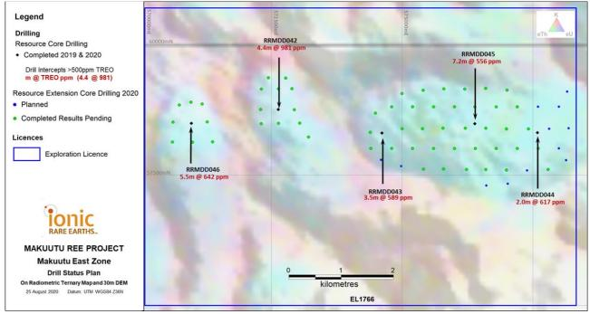
Figure 2: Current drill program showing both completed (green) and planned (blue) drill holes in the Makuutu Eastern Zone, EL 1766.
