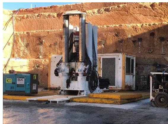
Raisebore on the fresh air intake/hoisting shaft collar
