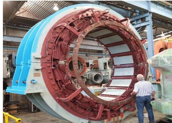
Shaft winder repairs (armature)
