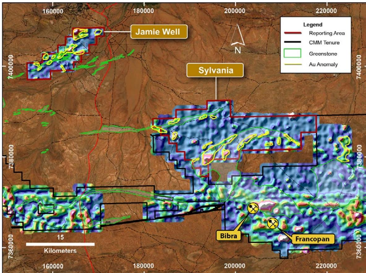
Figure 5: Soil sampling completed with identified geochemical targets
