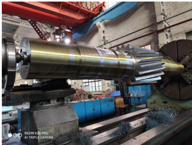
Ball mill head and pinion manufacture
