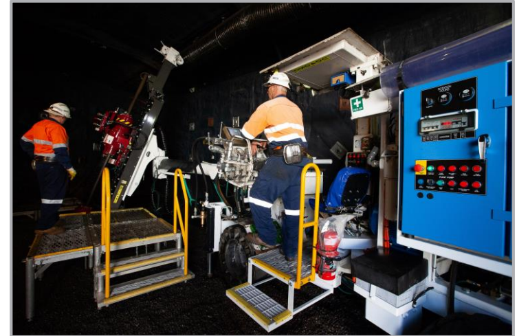
DeepEX prototype drill in use – capable of >2,000m diamond core holes from underground
