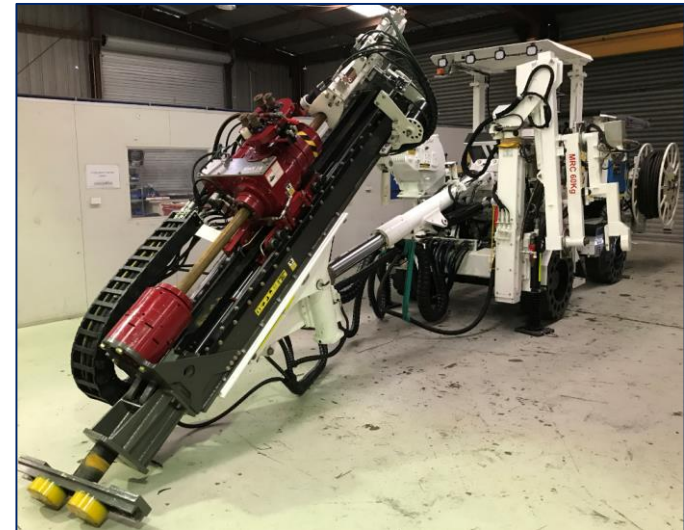
UD4501: First DeepEX build c/w rod handler
