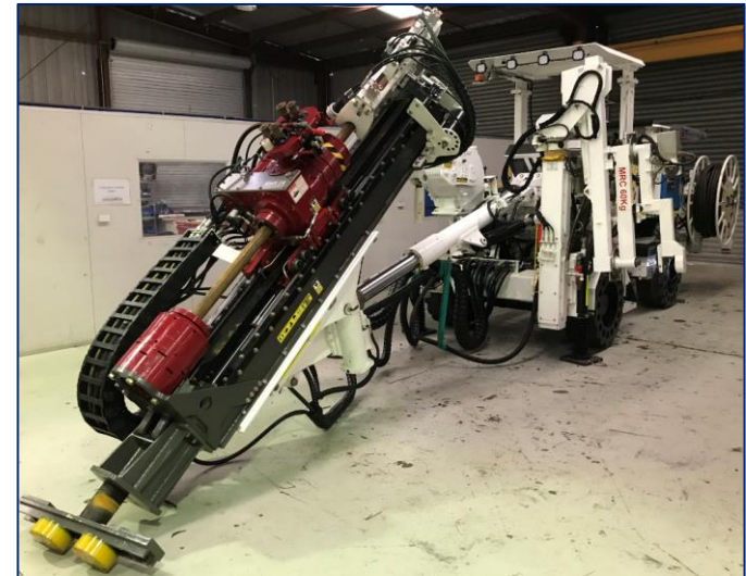
UD4501: First DeepEX build c/w rod handler
