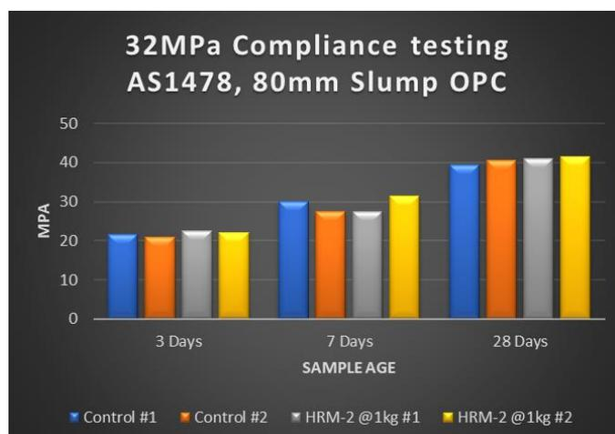
Figure 2 – Australian Standards Compliance Testing Progress
