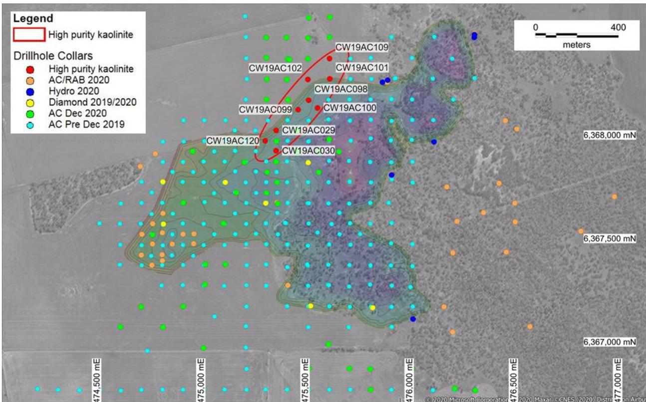
**Figure 5 – Great White drill collars with high purity kaolin coloured red, MGA Zone 53 GDA 94**
