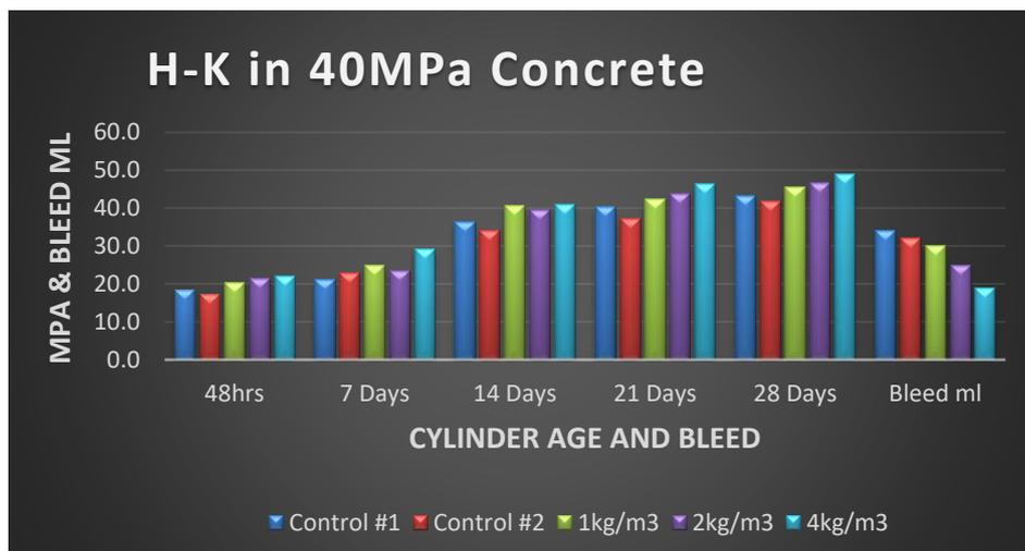
Figure 1 – Halloysite-Kaolin Results in 40MPa Concrete up to 28 Days
