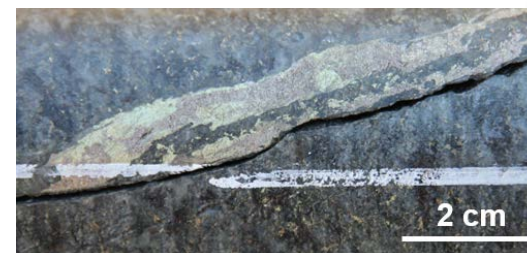
Late – stage pyrrhotite – chalcopyrite vein set with disseminated sulphide at 121.6m @ 121.6m
