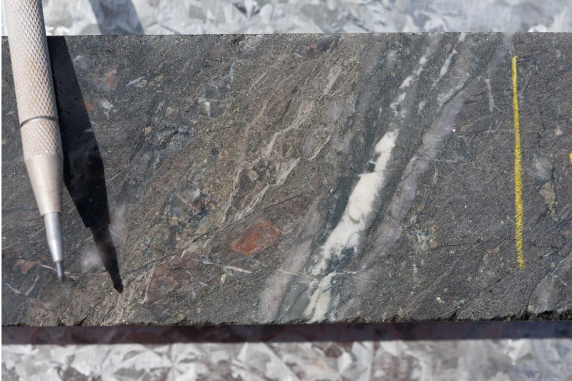
Figure 4: Foliation parallel quartz veining and sericite-silica-pyrite alteration
