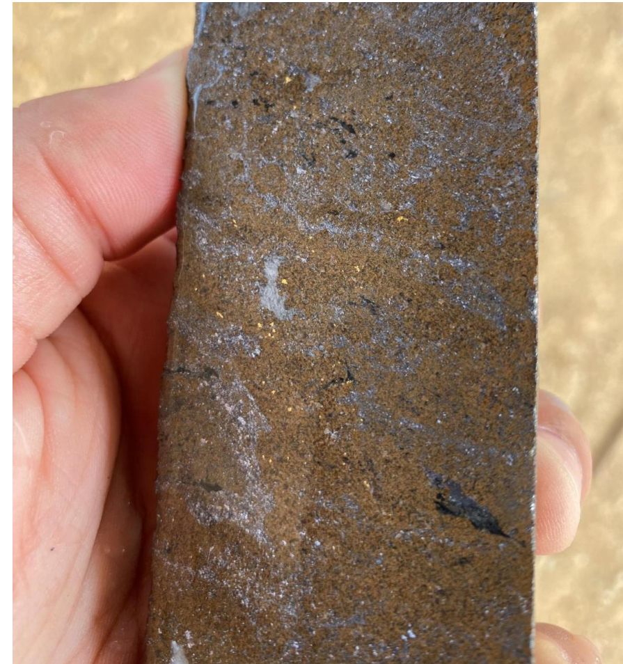
Massive sulphide mineralization from FDD107W1 comprising sphalerite (brown) and galena (grey) with abundant visible gold throughout (yellow). The photograph forms part of a one-metre interval grading 237g/t Au, 45.5% Zn, 19.8% Pb and 12g/t Ag.
