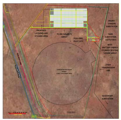
In the next quarter, a key focus is the grid connection studies to demonstrate GPS compliance to ElectraNet in an Application to Connect. Concurrently, Expressions of Interest are being sought for tenders for engineering and construction of the first stage of the project. This will provide firmer capital estimates for development of the project.
