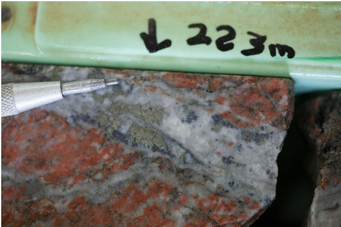
Figure 6: Low angle high grade (23 g/t) quartz-carbonate vein containing pyrite, sphalerite and galena
