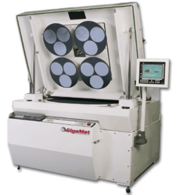
Capacity: 12, 150mm Wafers 4, 200mm Wafers
