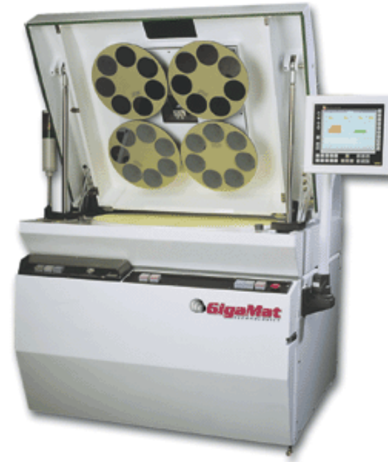
Capacity: 28, 100mm Wafers
