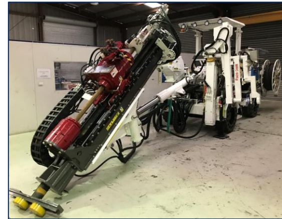
UD4501: First DeepEX build c/w rod handler
