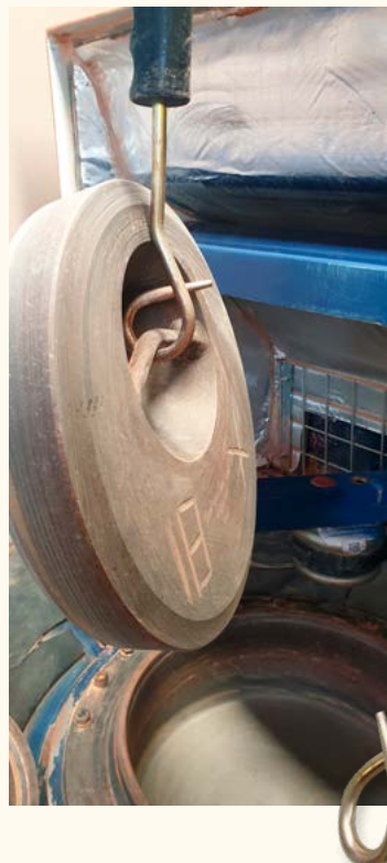
Piggy tail hook in operation
