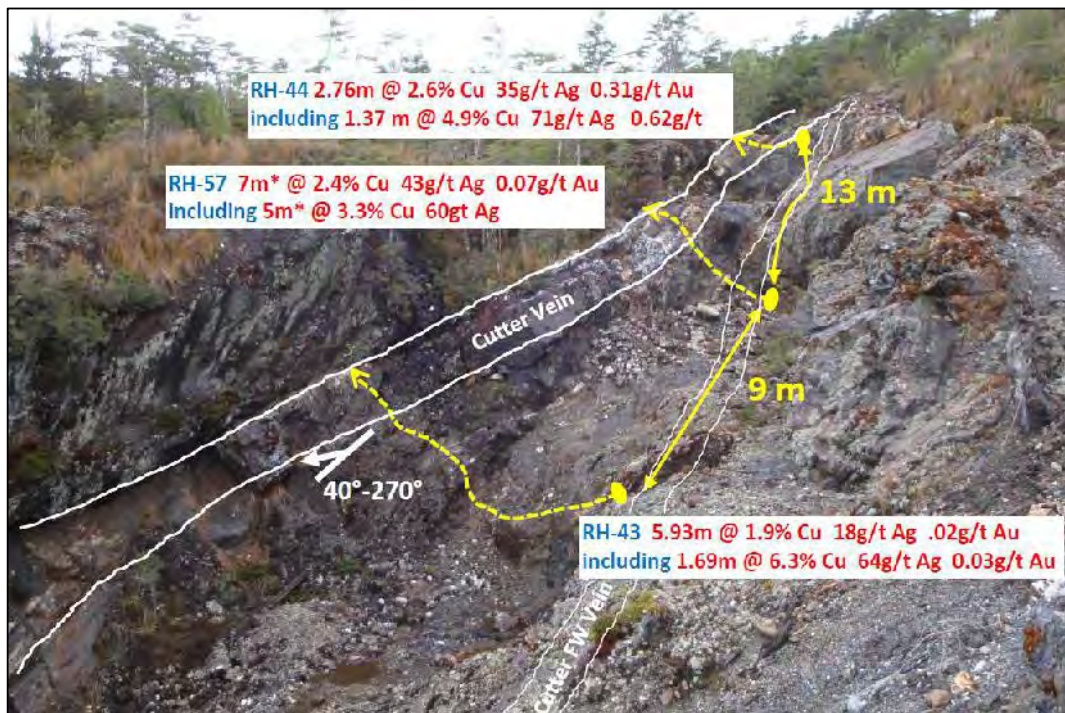
Figure 6.8 Photograph of Cutter open pit showing locations and grades of channel samples
