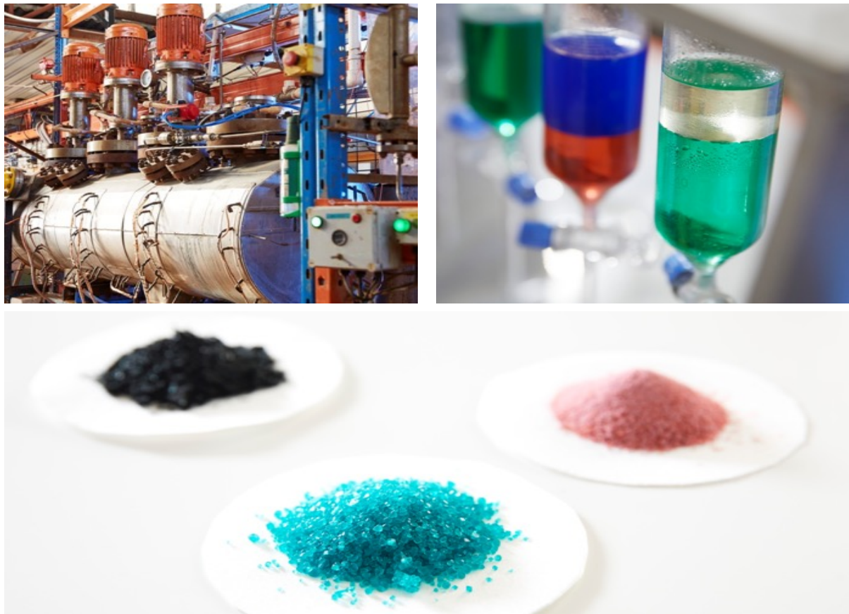
Figure 7: Collage of photographs taken of Australian Mines' demonstration scale processing plant in Western Australia, including images of the final cobalt sulphate (pink) and nickel sulphate (blue/green) and the intermediate mixed sulphide precipitate (MSP; black), which are routinely being produced.
