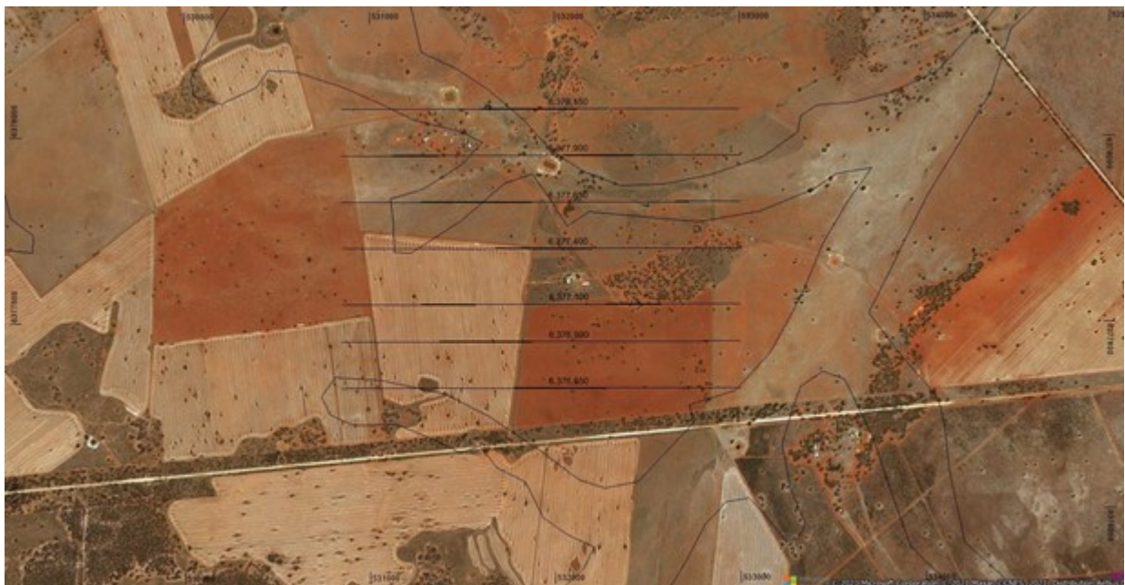
Figure 10: Survey lines of Australian Mines' Induced Polarisation (IP) survey overlain on aerial photo with outline of main drainage channels shown.
