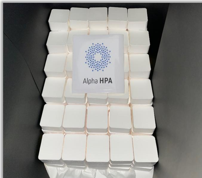
*HPA pellets for sapphire glass end users (pellet size: 45 x 45 x 20mm)*
