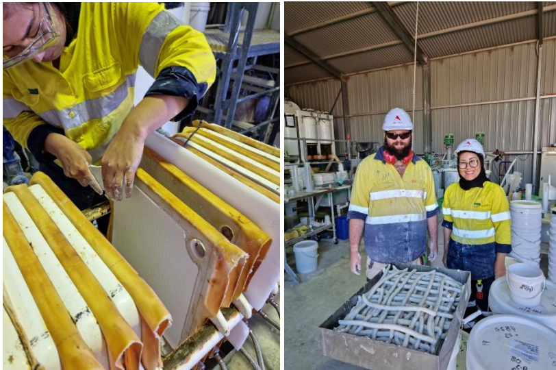
Figure 1 – Kaolin Refining at the Great White Project's Fully Equipped Pilot Plant
