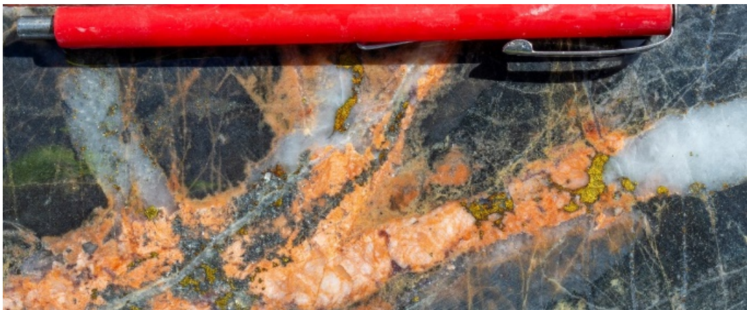
Figure 4. Multi-phase porphyry veins with blebby chalcopyrite mineralisation and associated potassic alteration overprinting volcanoclastic sediments, drill hole BD019-003 Central Porphyry, Briggs.
