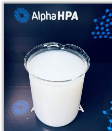
Sol-gel formation from high dispersible boehmite
