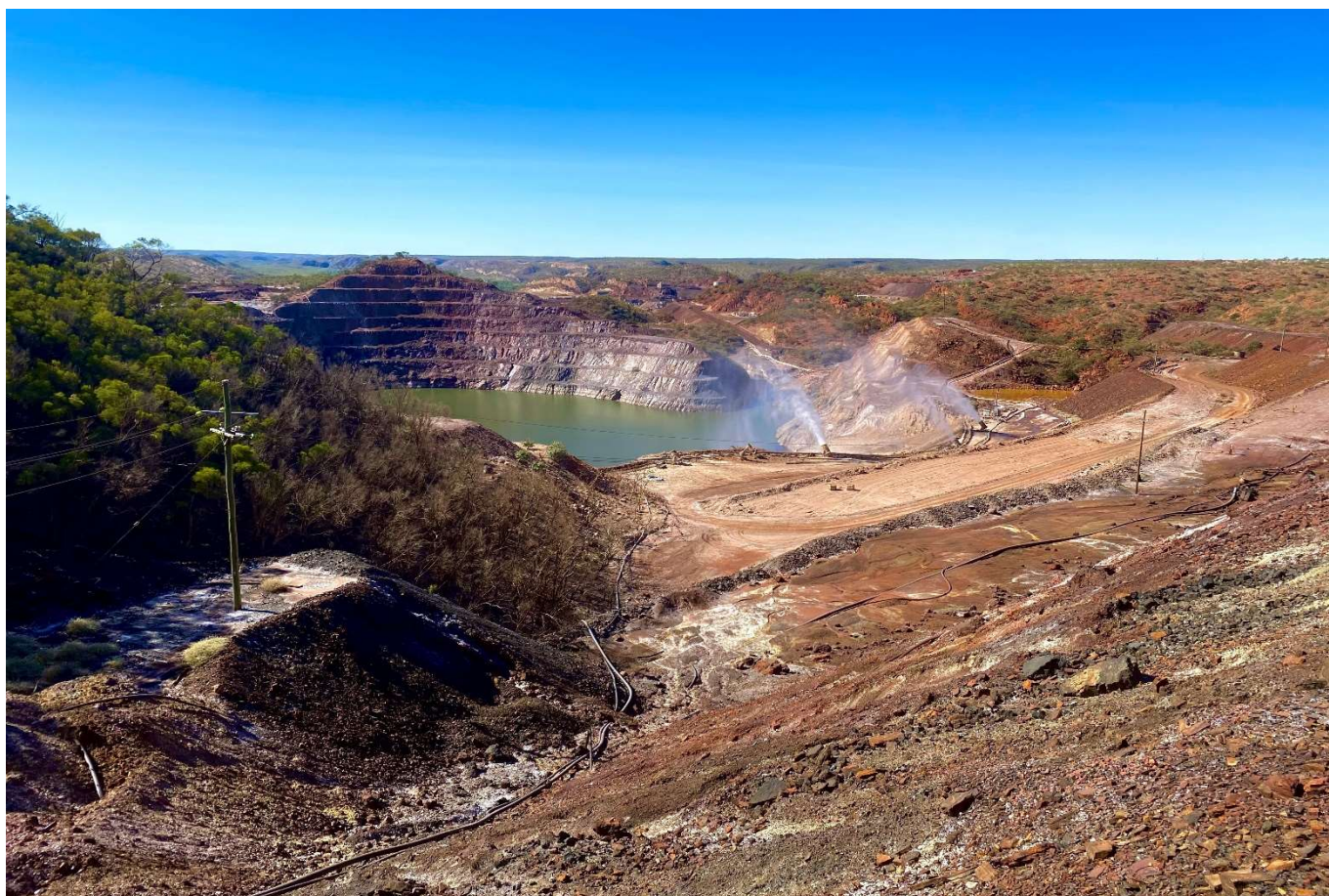
Evaporators in operation at Capricorn Copper
