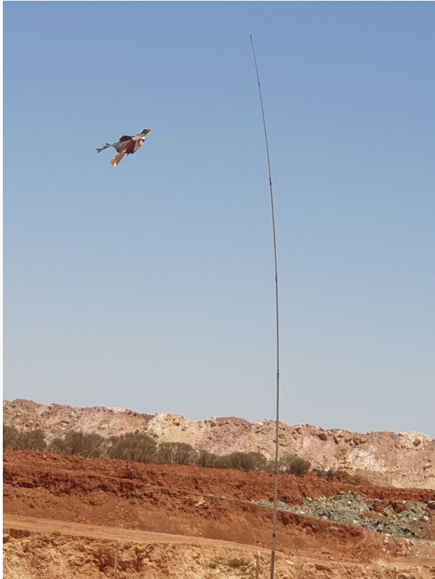
Figure 1: Bird deterrent kite
