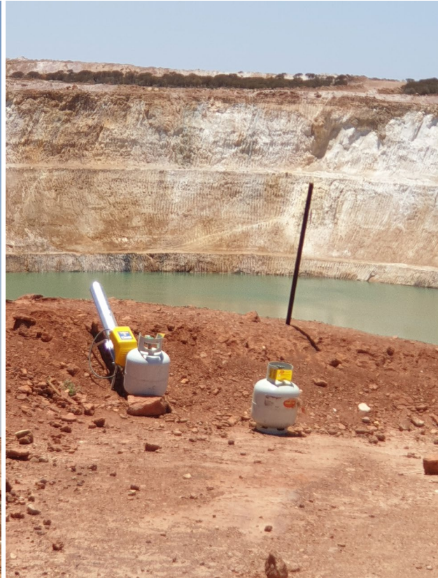
Figure 2: Gas powered noise deterrent
