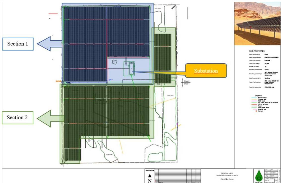
The Geotechnical assessment across the Site #1 area highlights a requirement to utilise different installation techniques across section 1 and section 2. The proposed configuration is based on a single axis tracking solution oriented North South to optimally track the sun. The relatively flat terrain across site #1 allows the design to utilise blocks of panels and trackers to be connected to a centralised string inverter and a mid voltage step-up transformer.
