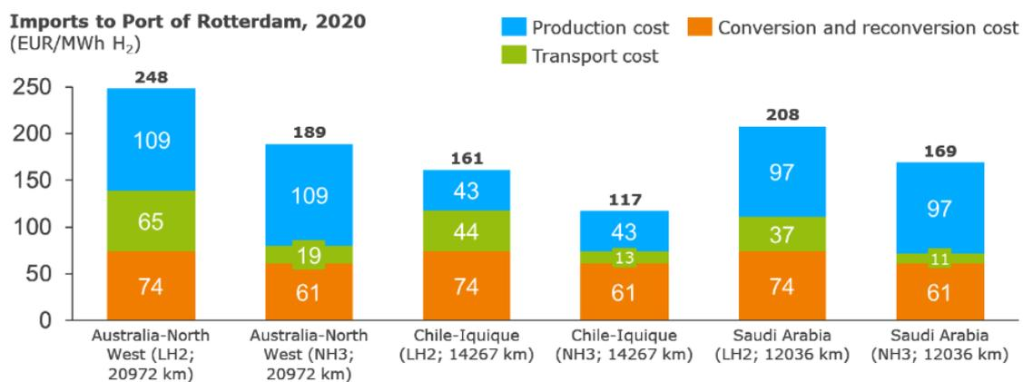
**Figure 25 Cost Estimates for Transport of Energy as Hydrogen or Ammonia<sup>27</sup>**
