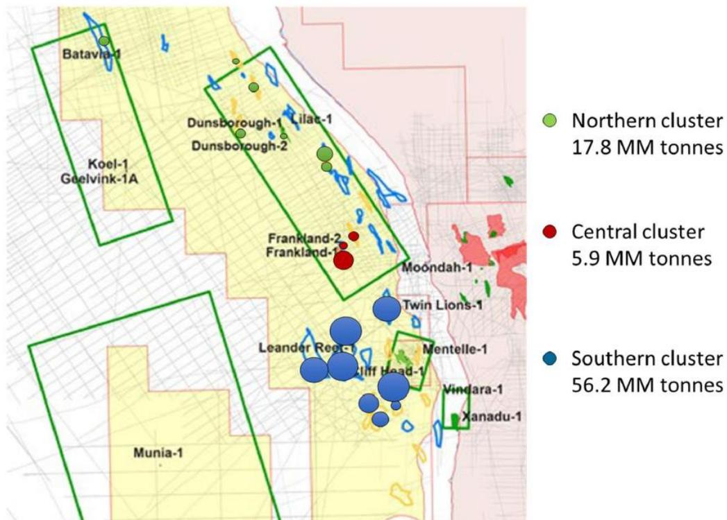
Figure 6 shows how the leads and structures within each of the clusters are situated in relation to a hypothetical series of three CCS project developments, with a development radius of 15 km from three central development locations.
