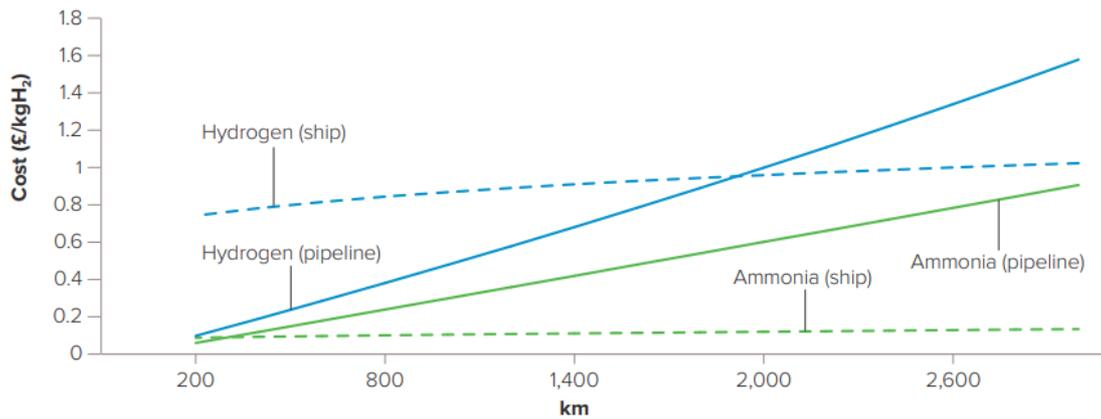
Note: Hydrogen transported via pipeline is gaseous and liquefied for shipping. Costs include both the transport and storage required; not the conversion, distribution or reconversion.
