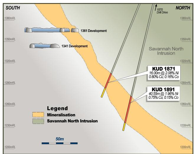
Figure 2: Oblique cross section at 6100mE +-30m grid showing drill holes KUD1871 and 1891 trace and proposed mineralisation model
