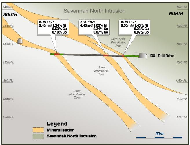
Figure 3: Cross section 6210mE showing drillhole KUD1827 and the three intersections through the multiple splays of the eastern margin of Savannah North
