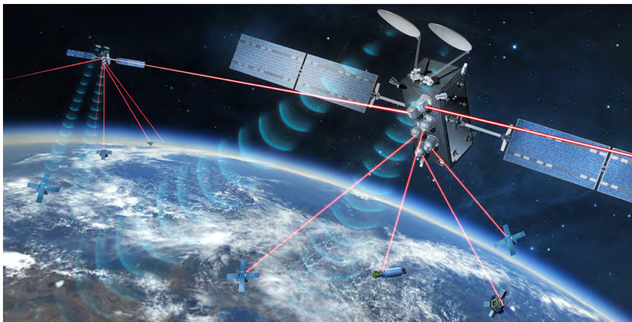
The SpaceLink relay satellites use optical links to transmit data between spacecraft on orbit and the ground
