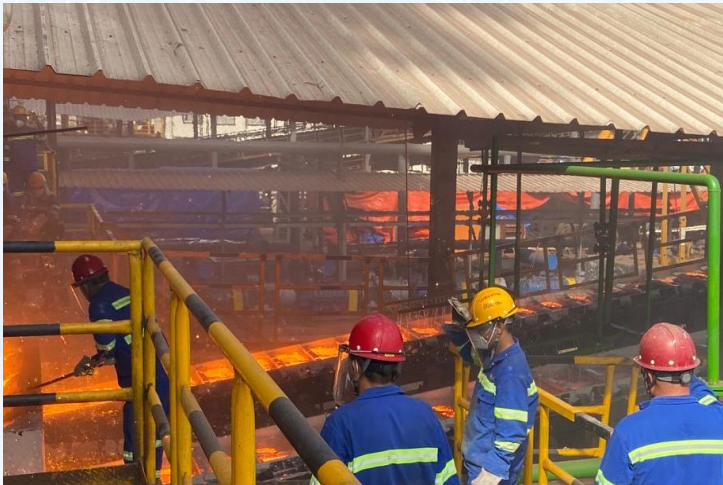
NPI being poured into an Ingot caster
