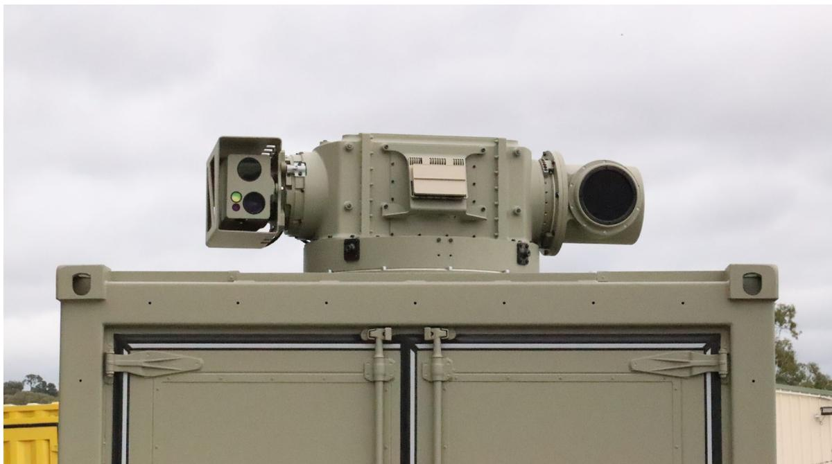
**Figure 1:** An operational DE beam director installed on a standard 20' container
