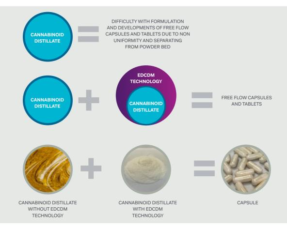
This novel matrix absorbs the distillate into a nano porous silicate particle where the distillate is effectively trapped in the structure of the silicate rendering the powder bed dry.
