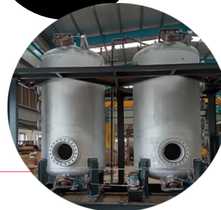
Carbon Capture Pilot Plant designed and manufactured (Height 5.0m)
