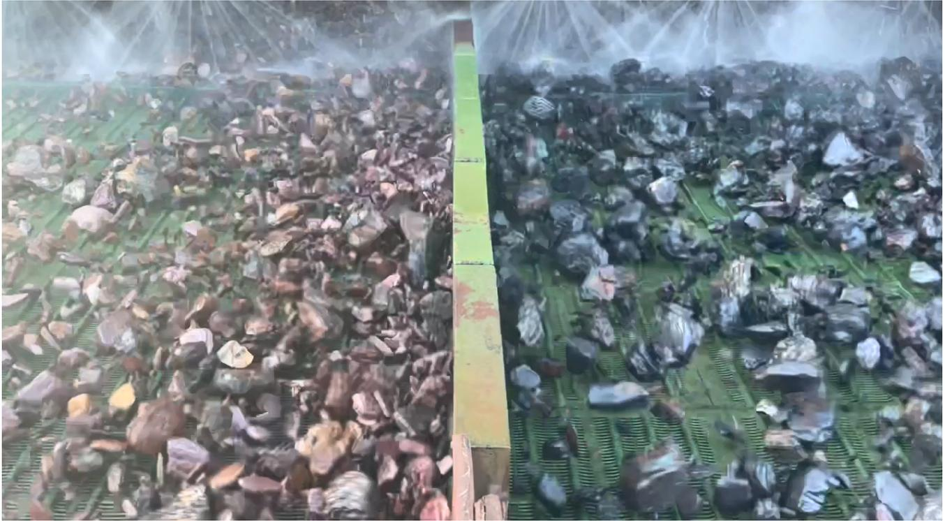
Figure 2. Butcherbird feed material on the wash screen after densimetric separation showing a clear delineation product and waste.
