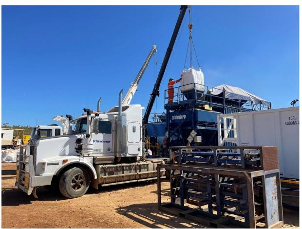
Loading proppant sand into the sand blender in preparation for a hydraulic stimulation
