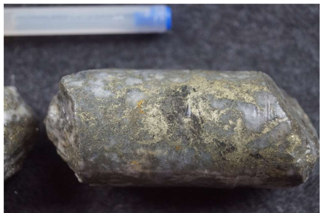
Left: Field crews operating portable small drill. Right: Example of the rock samples collected using portable small drill: Quartz Vein hosting chalcopyrite and pyrite mineralisation collected southeast of the Cristina Vein (Sample ID 5736 from hole CCL49-502)
