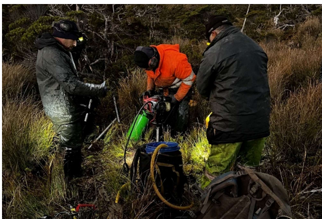
Left: Field crews operating portable small drill. Right: Example of the rock samples collected using portable small drill: Quartz Vein hosting chalcopyrite and pyrite mineralisation collected southeast of the Cristina Vein (Sample ID 5736 from hole CCL49-502)
