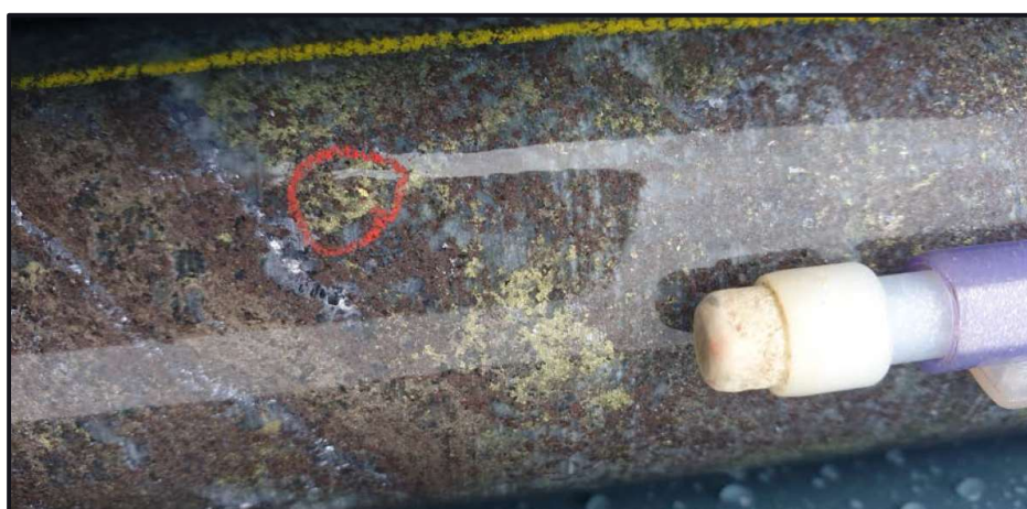
FDD177W10 – 539.9m : 1mm gold grain in massive sulphides (sphalerite, galena, chalcopyrite)
