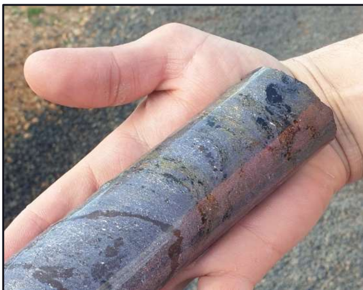
FDD184W5 – 504.4m : Massive sulphides dominated by galena, with strong sphalerite and chalcopyrite, and visible gold
