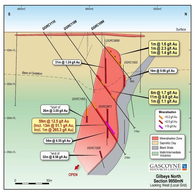
Figure 1: North-South cross-section on the 9950mN section through the "Never Never" lode showing the location of holes DGRC1099, DGRC1106 and DGRC1110 in relation to previously reported hole DGRC0971 (drilled east) and DGRC1026 (drilled north-east) as well as other nearby relevant intercepts.
