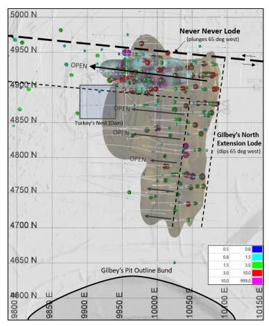
*Figure 5:* Plan view (3D software imaging) showing high grade intercepts so far and early wireframe interpretations. Note legend is drill interval (1m) grades in grams per tonne gold.
