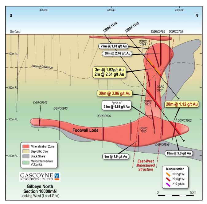
*Figure 2:* North-South cross-section on the 10000mN section through the East-West "Never Never" lode and the North-South Gilbey's North system showing the location of DGRC1108 and 1109 as well as previously reported DGRC1067 (drilled east) and other relevant intercepts.
