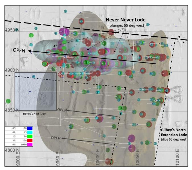
*Figure 6:* Plan view zoom showing high grade intercepts so far and early wireframe interpretations. Note that the latest drill-holes are yet to be included in the wireframe interpretations and appear to extend the current extents and legend is drill interval (1m) grades in grams per tonne gold.
