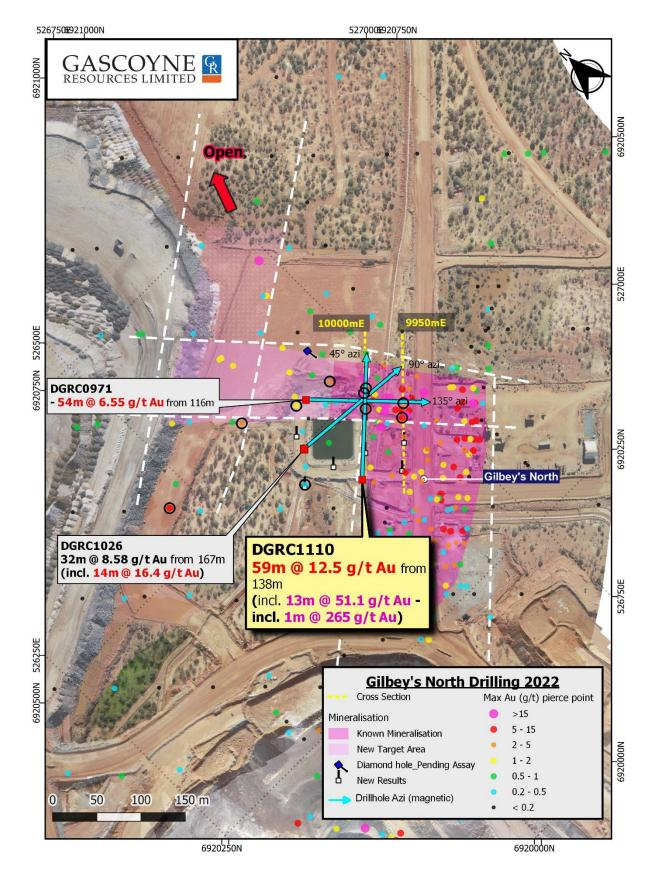
*Figure 3:* Plan view showing the location of recent RC drill-hole assays, the current schematic understanding of mineralisation in the Gilbey's North target area and the location of other nearby holes with assays pending.
