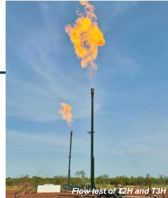
Tanumbirini 3H and 2H wells averaged 7.4 and 4.3 mmscfd, respectively, normalised to 1,000-metre lateral<sup>2</sup> over 8-days since recommencing flow testing in mid-August 2022 following installation of production tubing.
