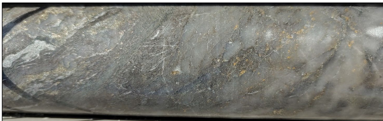
Figure 4: Abundant visible gold throughout NQ diameter core (roughly 2" diameter) from 397.5m downhole in drillhole DGDH032 from deep drilling of the high-grade Never Never Gold Deposit (assays pending).
