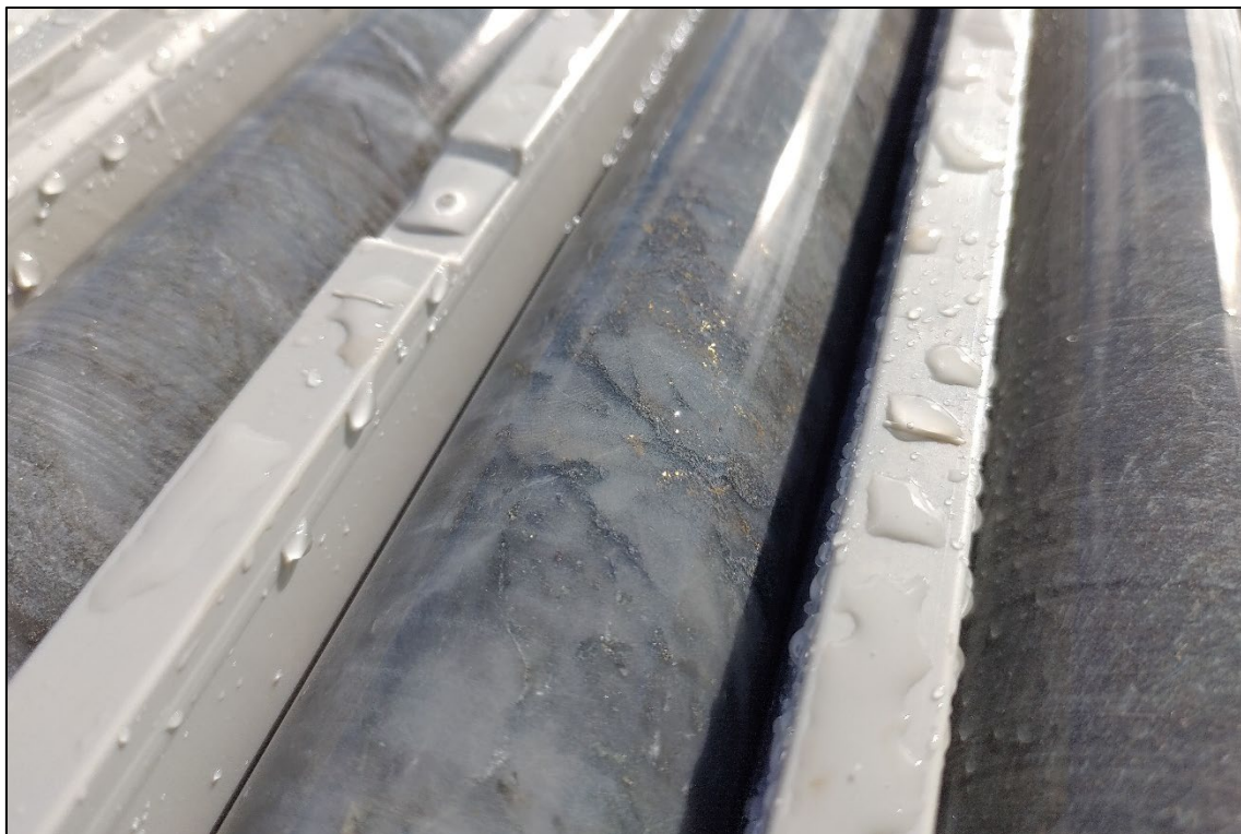
Figure 5: Visible gold in NQ drill core from 397.5m down-hole in DGDH032 (same interval as Figure 1, assays pending). The drill core displays the typical silica flooded textures and chlorite/sericite/biotite/carbonate alteration seen in all previous Never Never Gold Deposit intercepts.
