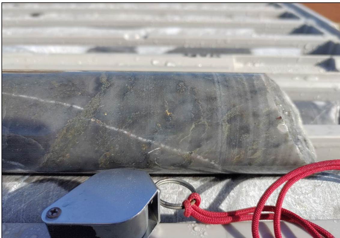
Figure 6: Coarse specks of visible gold in DGDH032 from 398.5m downhole in NQ diameter core from deep drilling of the high-grade Never Never Gold Deposit (assays pending).
