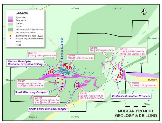
Figure 2: Moblan drillhole plan view with selected drill intercepts
