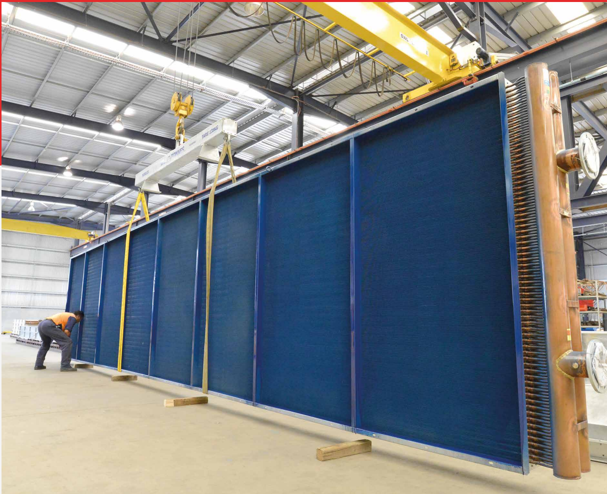
Air Radiators Industrial (Gillman, SA) manufactures large radiators to cool diesel and gas engines in power generation stations.
