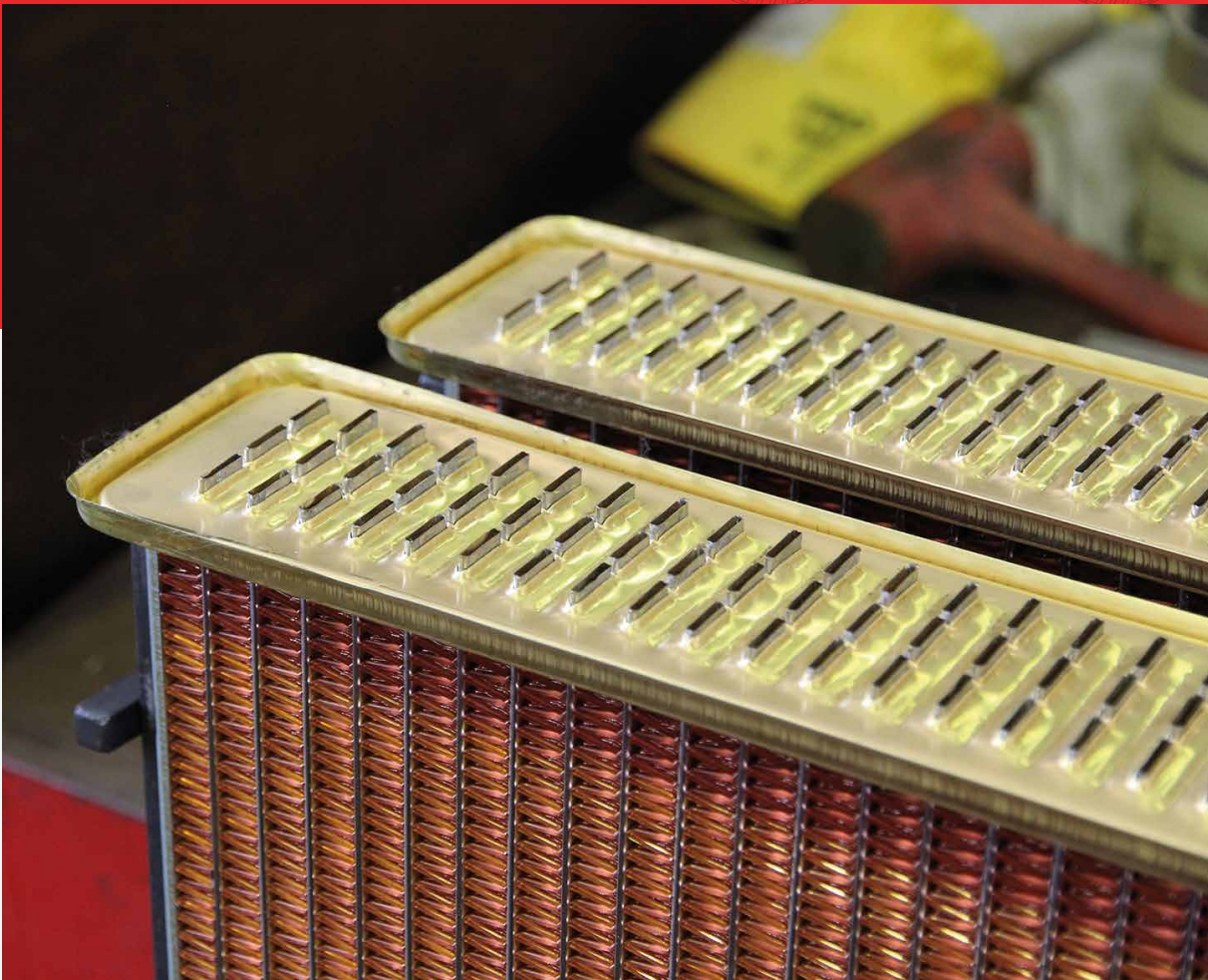
Brass header plates fitted to Adrad 3-row automotive copper cores (Beverly, SA) during assembly.
