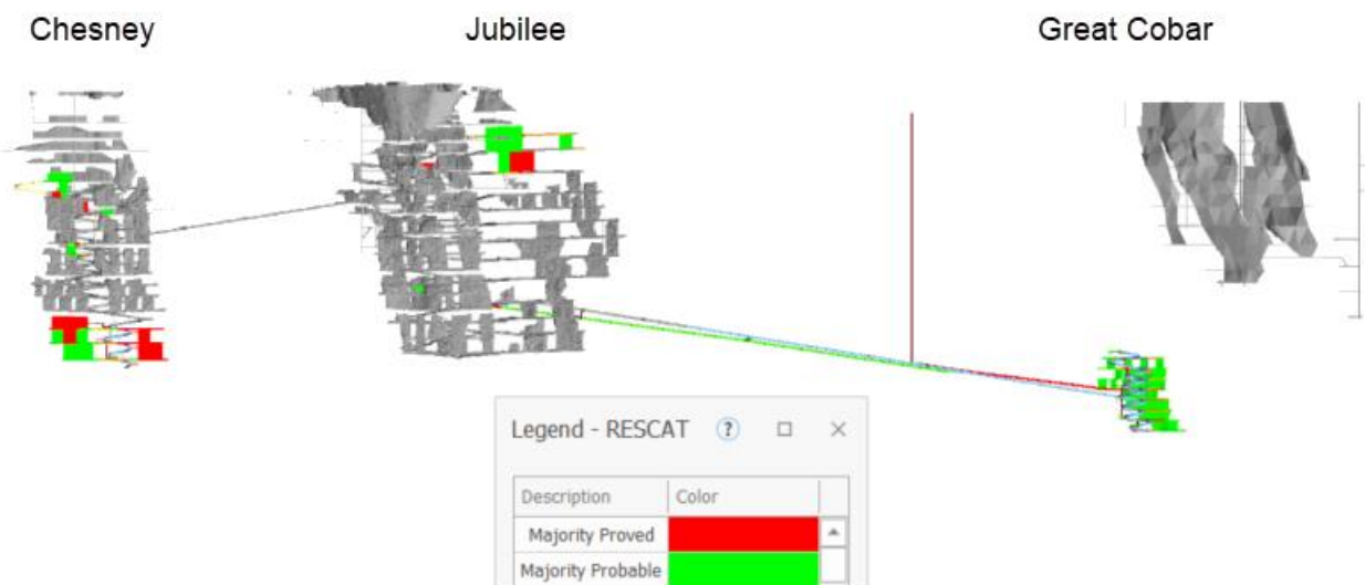
Figure 7. Long section facing west of the Peak North Mine showing Proved (red) and Probable (green) Ore Reserve classifications.
