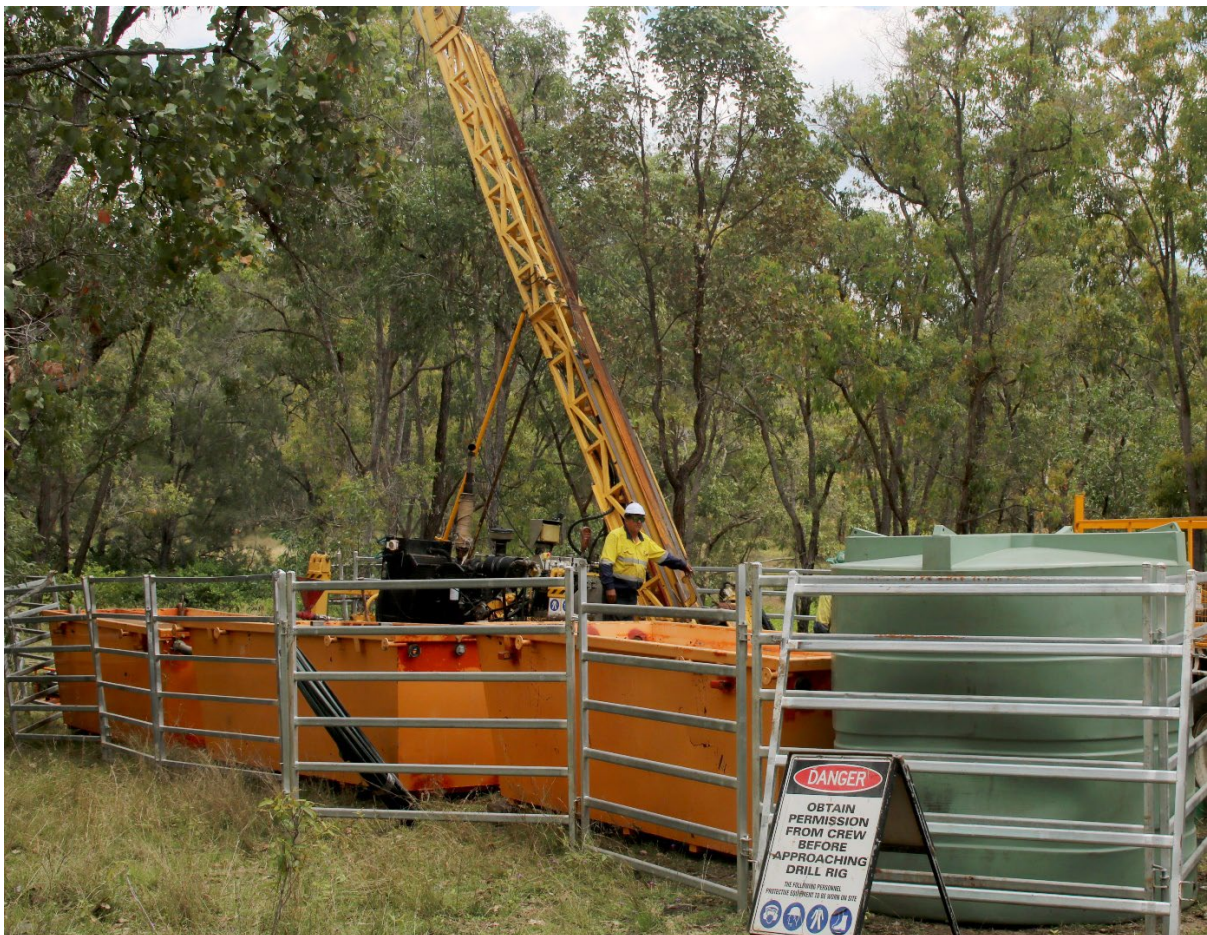
Figure 1. Core drilling rig during initial set-up for the first core hole into the northern porphyry target at Briggs
