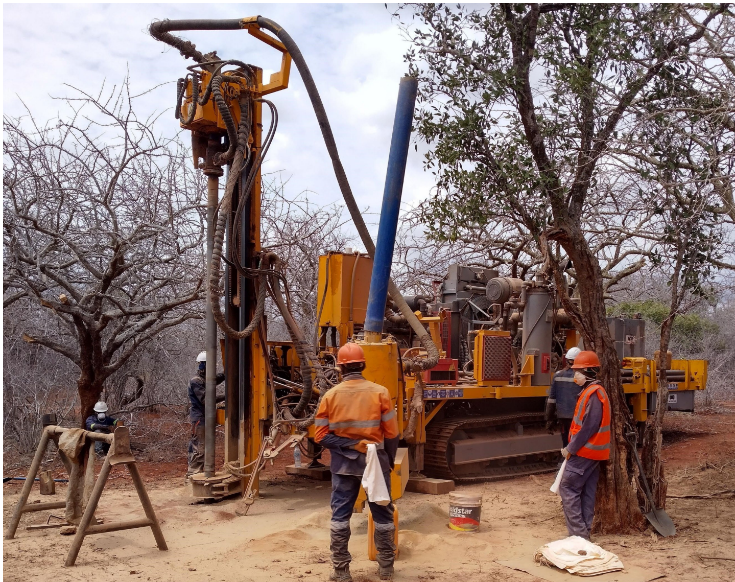
Figure 1: Reverse circulation drill rig in Tanzania.
