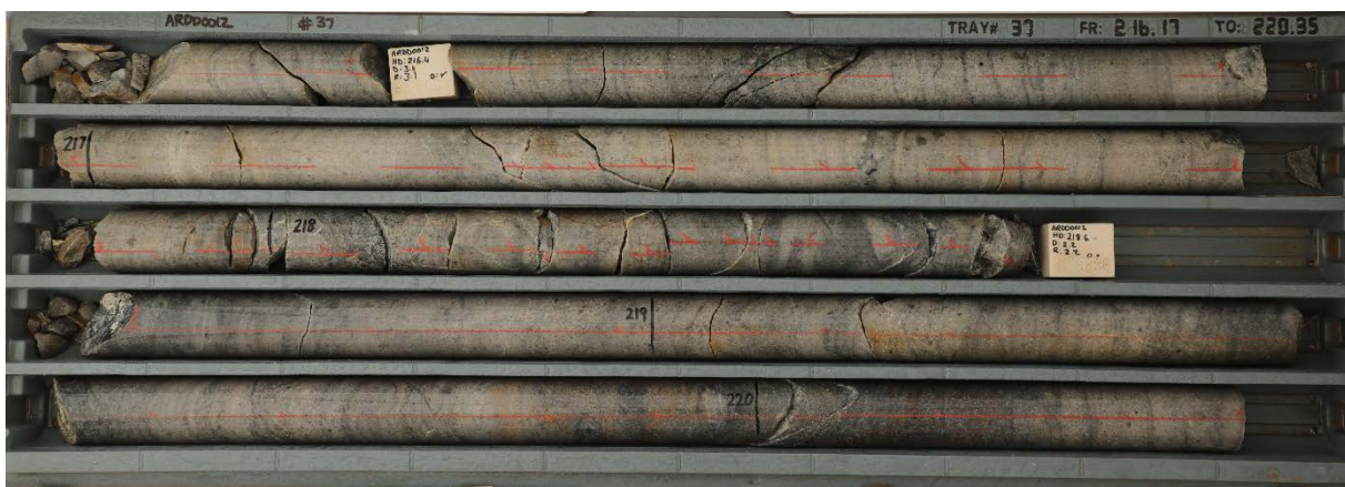
Figure 3: Disseminated primary uranium mineralisation in bleached and pyritic Mamadawerre Sandstone in drill hole ARDD0012 (downhole interval from 216.17 to 220.35m).
