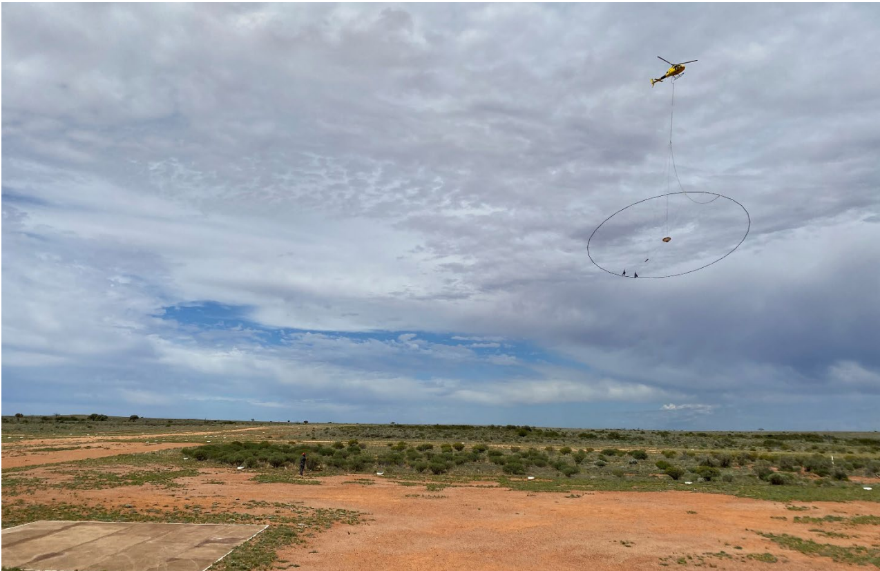
Figure 1: HelITEM 2 conducting the AEM Survey
