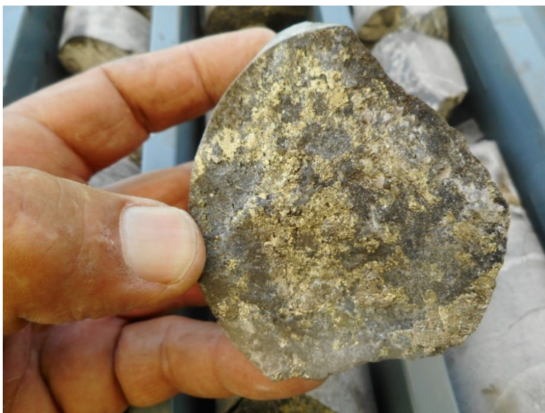
Figure 5 Coarse chalcopyrite associated with porphyry-style quartz vein. Drill hole 22BRD0013 at ~86m.
