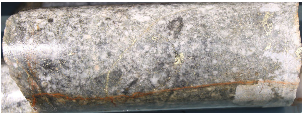
Figure 7 Coarse chalcopyrite veins and disseminations in porphyritic granodiorite. Drill hole 22BRD0013 at ~434m down-hole depth. HQ3 core (63.5mm diameter).
