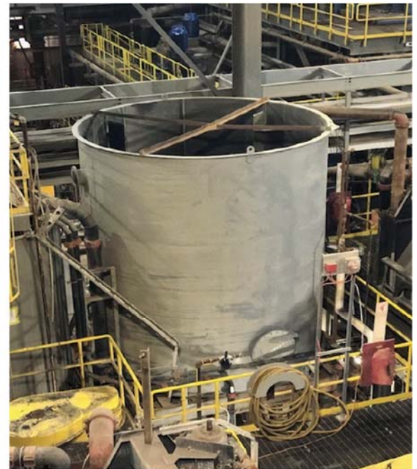
Left: Derrick Screens ready for electrical installation; Right: Conditioning tank in place for full installation
