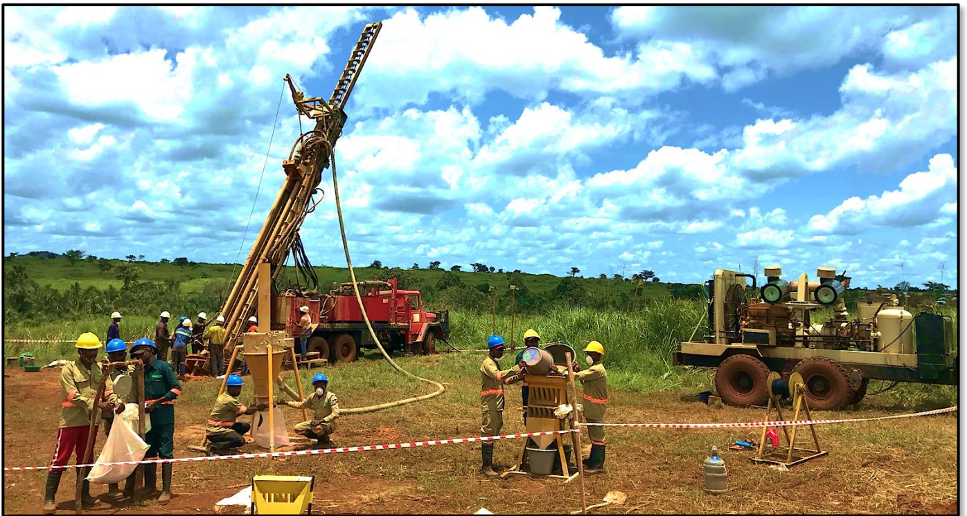
Figure 2 - RC Rig and Drill Crew at Kebabigada South East
