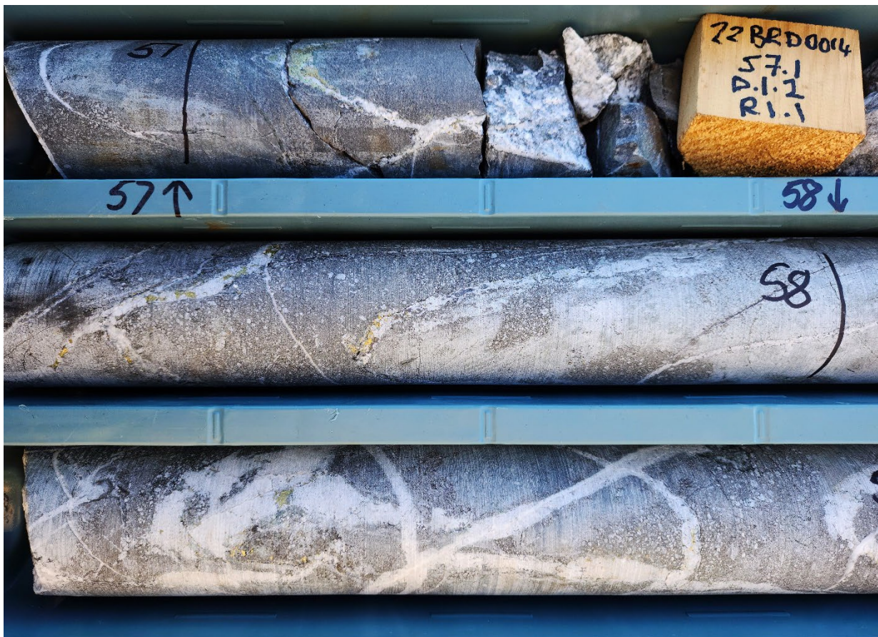
Figure 5 Quartz-chalcopyrite porphyry-style veins with minor chloritic alteration in porphyritic volcaniclastic host rocks. 22BRD0014 at 57-59m down-hole depth.
