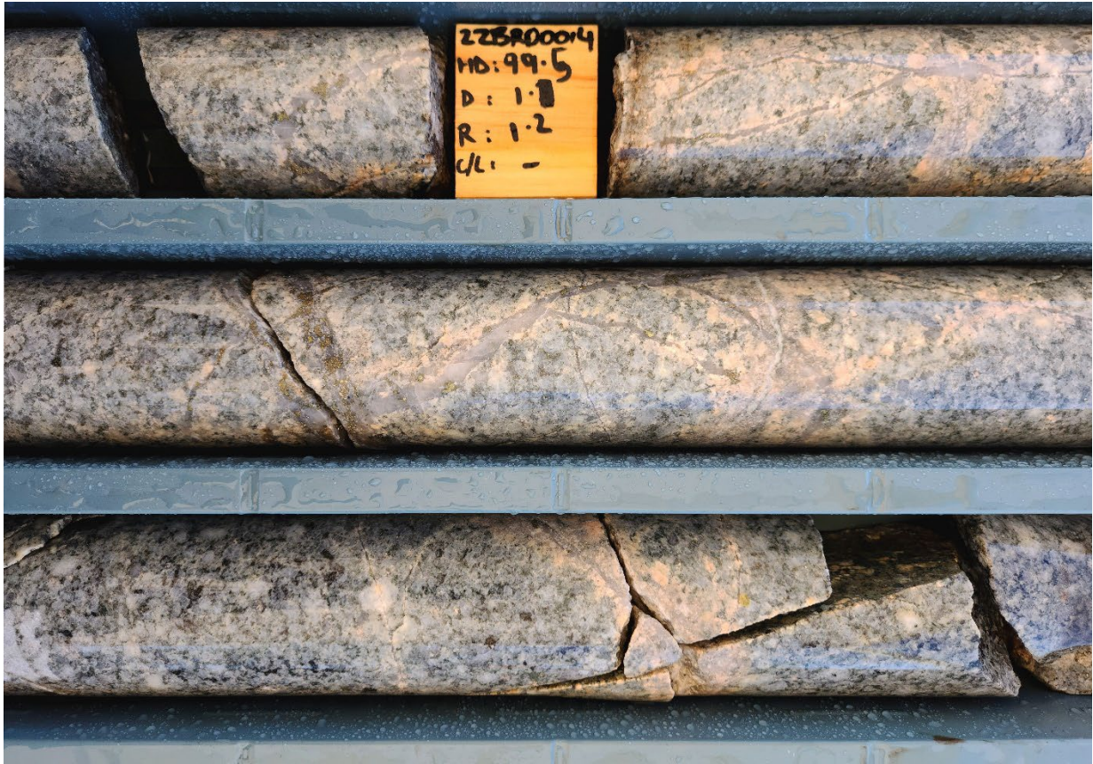
Figure 6 Porphyritic granodiorite cut by numerous quartz-chalcopyrite porphyry-style veins with orthoclase (potassic) alteration haloes. 22BRD0014 at approximately 100m down-hole depth.
