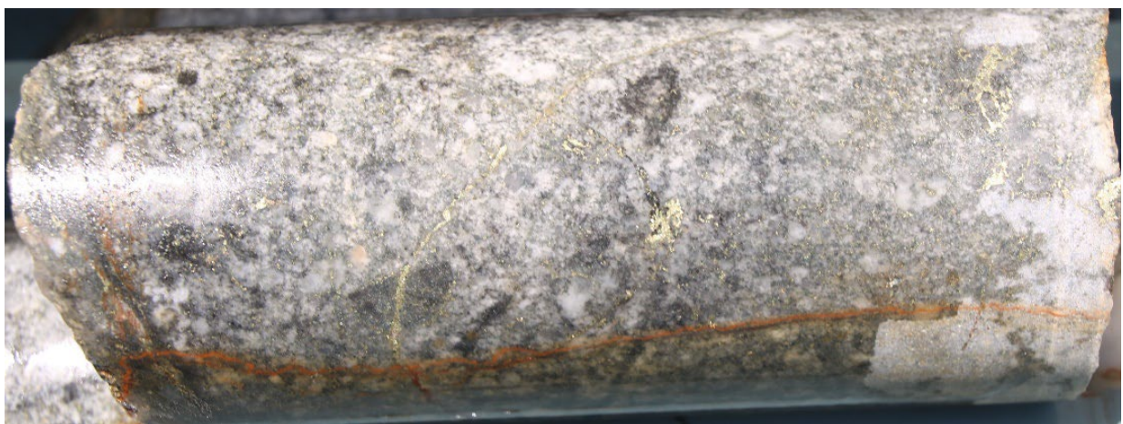
Figure 4 Coarse chalcopyrite veins and disseminations in porphyritic granodiorite. This photograph is from a 2m sample assaying 0.75% copper. Drill hole 22BRD0013 at 434m down-hole depth. HQ3 core (63.5mm diameter).
