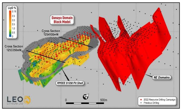
Figure 1: Oblique view of the updated Danaya Domain Block Model and the geological model of the NE-Domains. Block Model Li2O grade shown and coloured by grade. NE-Domains in red. US\$1250 RPEEE pit shell shown in grey. Only material above the pit shell is reported as Mineral Resource.
