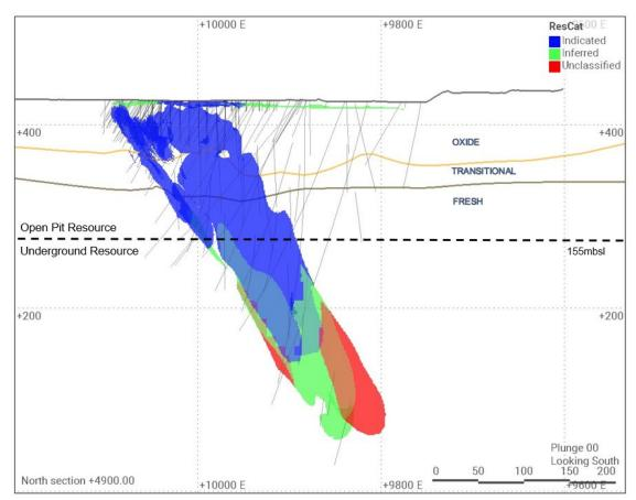
*Figure 3:* Section 4,900N (+/-50m) looking south through the Never Never Gold Deposit illustrating Resource Category (ResCat) and drill hole traces
